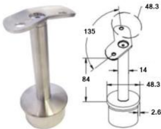
48-HH1005-135 135 Degree Saddle (In part form) 304/316
