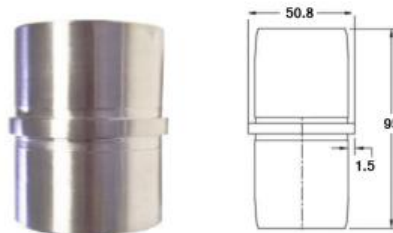
RV1001-50.8x1.5mm Straight Connector 316
