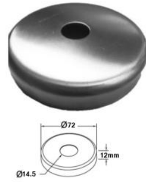
CP-76 Handrail bracket cover plate
