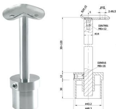
48-HH1005-ADJ-90 48.3 x 2.5mm Wall 90 Degree Saddle 316 Satin Finish
