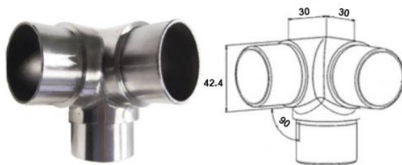
EVB1009-42.4MM 3 Way Corner Connector 304/316
