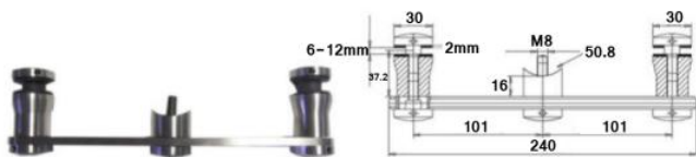
GLH1010K-30-50.8 Double Glass Retainer 316
