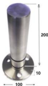
BDH1005/100/50.8 200mm Spigot and 100mm Plate - 3 x M13 Fixing Holes 304/316
