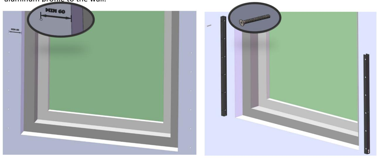
**Step 2.** Install the L shape cladding onto the aluminum profiles.
