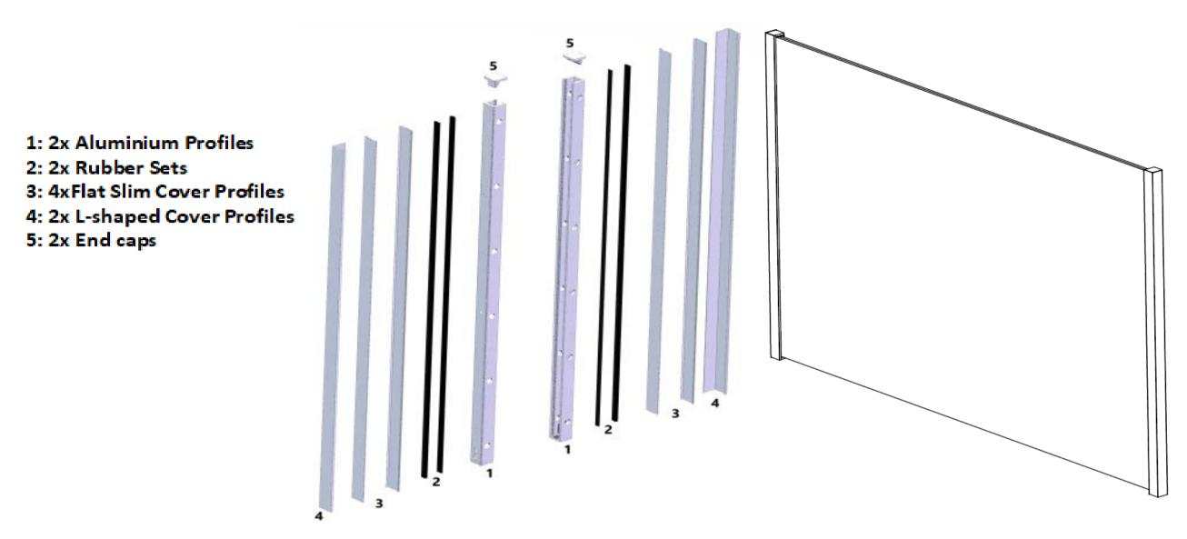
**Step 1.** Use drill bit to predrill holes for drop in anchors or screws (depending on the substrate), fix the aluminum profile to the wall.
