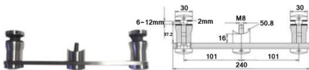
GLH1010K-30-50.8 Double Glass Retainer 316
