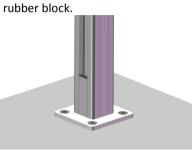
Step 3. Install and insert the outside rubber strip along the slot on the post.
