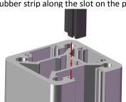
Step 7. Drill and screw the handrail to the post with the drilling tool (removed afterwards).
