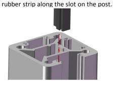
Step 3. Install and insert the outside
