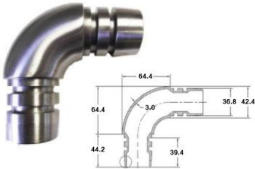
MS1008-42.4x2.6mm 90 Degree radius tube connection
