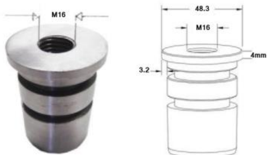
MS1060 - 48.3 x 3.2mm Top insert for 16mm stem
